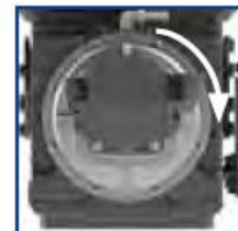
Version HFR Group 4 108,9 cc/rev - Pmax 250 bar - In G 1" - Out G 1" 1/4
